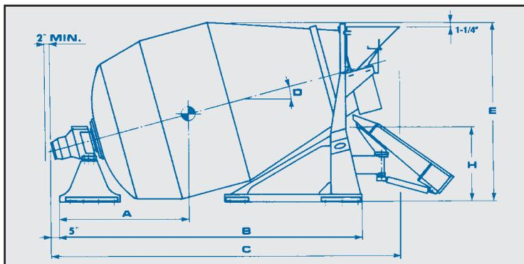
**DRUM:** 1/4" spun drumhead; 48" inside reinforcing plate; 3/16" SAE 1524 wear resistant ( high manganese, low carbon ) steel drum shell welded 100% inside and out; 3/16" SAE 1524 blades with hard surfaced lips; solid wire welded seams; solid steel drum track machined inside taper and out square; 43" discharge opening; auxiliary surge fins; 16" X 22.5" bolt on oval inspection hatch.
