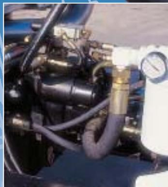
*Eaton heavy duty series hydrostatics provide high torque capability for efficient loading, mixing and discharge of low slump concrete. An "A pad" pump provides reliable power for the main chute.*
