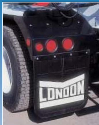
*The standard lighting system utilizes Trucklite sealed lights, junction box and harness. Optional dual tail lites shown.*
