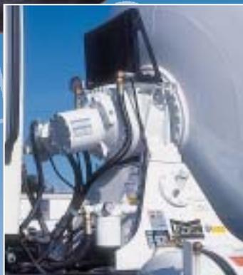
*The mixer drum is driven by a ZF PK7500 planetary direct drive gearbox providing over 53,000 ft.lbs. of torque. A 15 gallon oil tank is incorporated into the front pedestal.*
