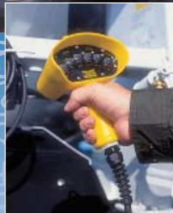
Rear pendant on 20 ft. quick disconnect cable incorporates control for mix/discharge, engine throttle as well as optional air chute lock, chute lift, air lift hopper and drum pause/resume.
