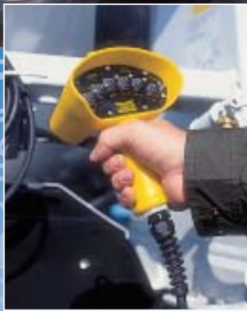
Rear pendant on 20 ft. quick disconnect cable incorporates control for mix/discharge, engine throttle as well as optional air chute lock, chute lift, air lift hopper and drum pause/resume.
