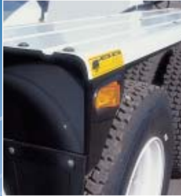
Roll formed fenders are available in steel and aluminum. Light weight poly fenders are also available. Mid-ship combination signal/clearance lights are standard.
